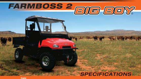
Engine Type DIAHATSU - 3 Cylinder, Water & Oil Cooled 1.0L Diesel
